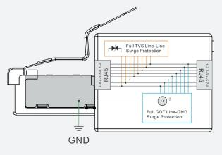
**Note:** The metal release tab does not provide a ground connection. Ground connection is made by connection with the metal sides as shown in grey in the diagram with green GND connection.
